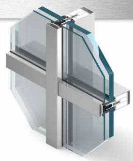
MB-SR50 El is a "stick-build" mullion & transom curtain wall system, designed for the construction of fire-proof screens & facades. Used conventionally for all typical & the most challenging of designs & building requirements, the system has achieved classifications El15, El30, El45, El60 according to the standard BS-EN 1364-3. The system has been classified as non-fire-propagating (NFP). All standards attained have been approved by EXOVA, Warrington, as UK market compliant (Reg. No. 195772).
