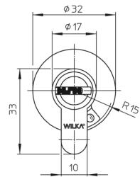
**Profil-Knaufzylinder****Profile knob cylinders****1407 / 3607****Knaufzylinder kurz / Knob cylinder short**
